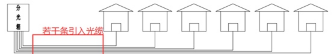
Figure 1 Traditional FTTH construction
